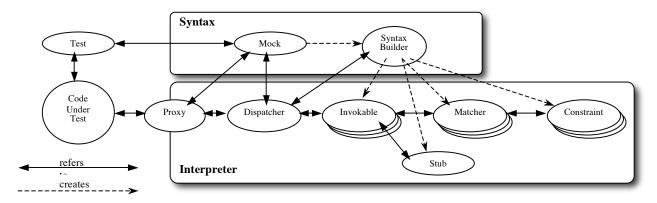
Figure 2. jMock Syntax and Interpreter layers
